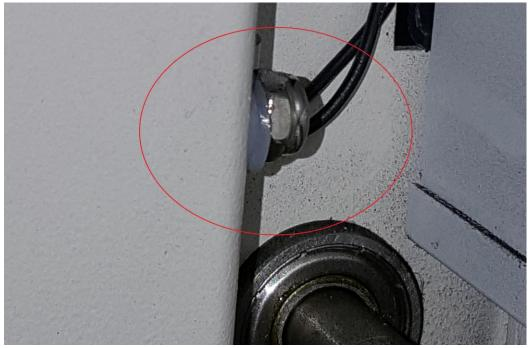
4. Unscrew the 2 screws holding the interlock in place to remove
