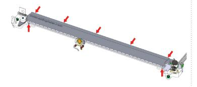
6. Remove 5/64" Hex screw on Auto Focus Plunger magnet. Do NOT discard the magnet.
