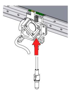
9. While applying light pressure upwards on plunger, reattach the magnet with 5/64" Hex screw. The magnet must face towards the back of the machine.
