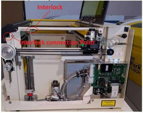
2. Disconnect Interlock from Wiring Harness
