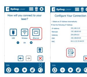
6. Select **Use the following IP Address**. In the IP Address field enter **192.168.3.10** This is the standard IP address for direct connection.
