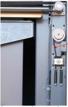
Unhook this belt to release the motor from the pulley system
