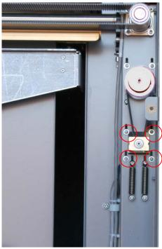
7. Disengage the small belt connected to the motor pulley from the large silver spindle above the motor.
