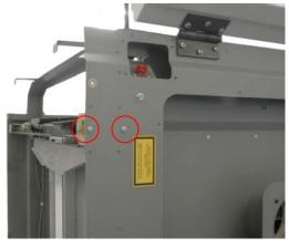
b. Loosen the four screws on the Y-belt bracket.
