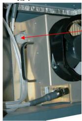
Use a small flat head screw driver to loosen the two screws
