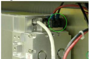
4. Disconnect the eight pronged electrical connector found above the power supply.
