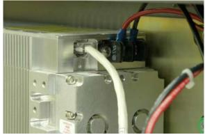
3. Loosen the screws holding the positive and negative ground wires on the laser. Remove the wires.
