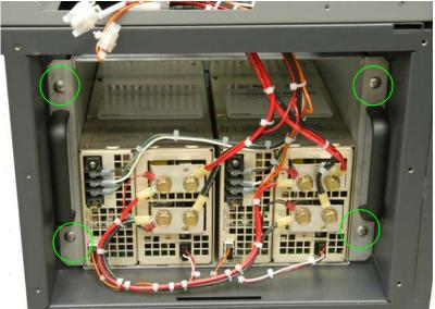
6. Using the handles, slide the power supply out of the machine.
