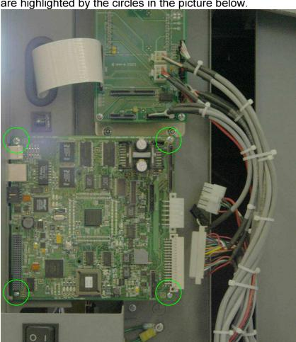
7. Remove the controller board, replace with a new controller board and tighten the four screws on each corner of the controller board.
