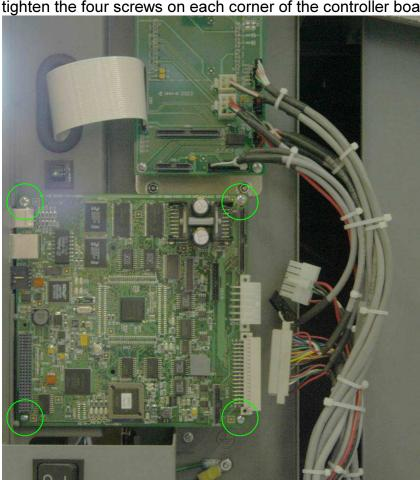
8. Reconnect the five connectors to the controller board.
