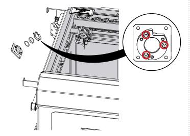
11. Install four (4) Phillips head screws on mirror plate.
