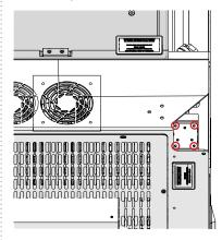
15. Install window optic with three (3) 3/32" Hex screws.
