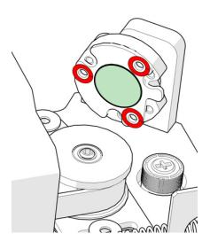
There are adhesive gaskets between the mirror plates and orange periscope. To remove these, you may need to gently pry the plate away from the periscope. Before removing these, label the top of each plate.
