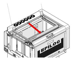
3. Locate mirror on end of X-Axis rail.
