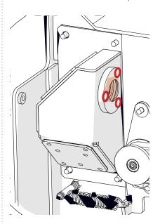
3 Remove four (4) Phillips head screws on mirror plate.
