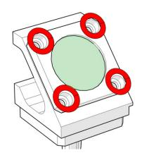
12. Align lens assembly and install two (2) 3/32" Hex screws.
