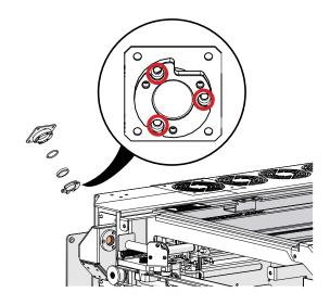
14. Install four (4) Phillips head screws on mirror plate.
