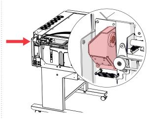
2. Remove three (3) 3/32" Hex screws to access the window optic.
