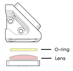
7. Install replacement lens with curved side facing up.
