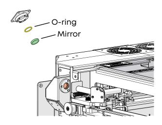
6. Remove four (4) Phillips head screws on mirror plate.
