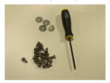
The screws will be used to assemble the stand and the washers are used to attach the stand to the machine. There should be two extra screws when assembly is complete.
