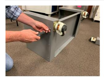
Install three of the screws on the outside wall of the Wide End Cap, attaching the End Cap to the Shelf.
