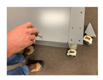
Connect the Rear Casters using 4x screws for each Rear Caster.
