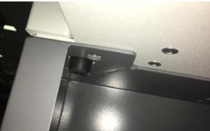
Reach inside the Stand and remove the rubber feet from the laser system. Remove the fastener from the rubber feet.
