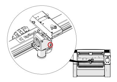
2. Slide optics cover up and tighten top left thumb screw to hold the cover in place.
