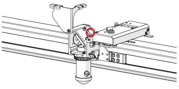
5. Close optics cover and secure thumb screws.
