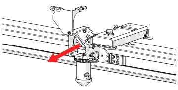
5. Remove the rubber air assist tubing from the lens tube.
