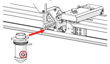
2. Insert manual focus gauge into holes on lens clamp and turn to the right.
