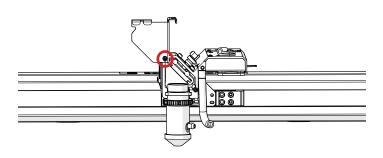
3. Loosen the large thumb screw holding the mirror.
