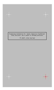
9. Once the last target is pressed, the engraver will return to the Advanced Settings menu. There is no success message for this calibration procedure.
