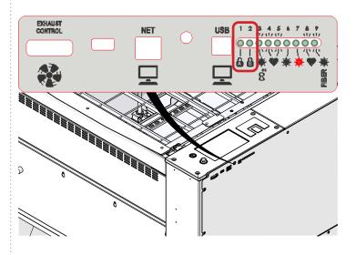
2. The two interlock LEDs are labeled with lock icons. These LEDs must be illuminated when the doors are closed.
