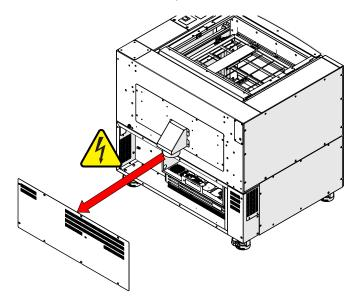
3. Remove the mirror 1 cover located at the bottom left corner of the machine.
