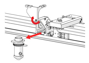
2. Remove the carriage mirror. Clean and check for damage.
