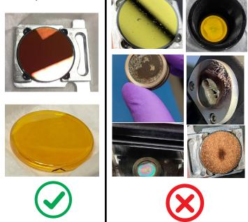
1. Remove the lens assembly. Clean both sides of the lens and check for damage.
