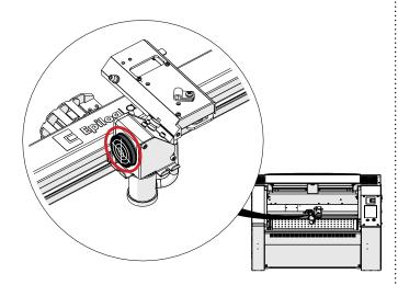
2. Jog the carriage to Top Left (home position). Turn on the red dot pointer. Verify the red dot is within the center ring of the target.
