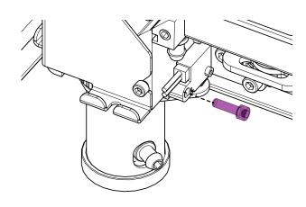
9. Install adapter plate between replacement autofocus switch and carriage assembly.
