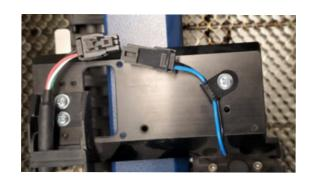
14. Install Phillips screw to secure harnessing.
