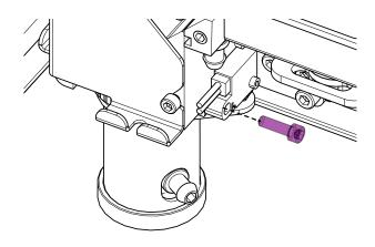
9. Install adapter plate between carriage assembly and replacement autofocus switch.
