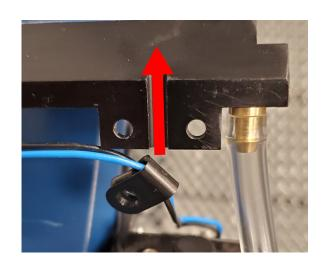
12. Install two (2) T 10 Torx screws.
