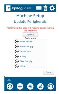
When running a peripheral update, do not power off the engraver. During a peripheral update it is common for the display to power off. Once the update has been applied, the engraver will prompt to restart.
