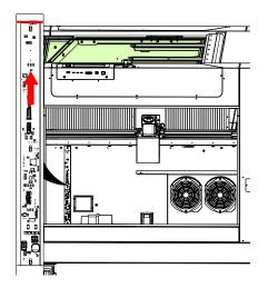
4. Tighten the four (4) 5/16 nuts that secure the z-axis PCB to the engraver chassis:
