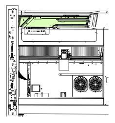
6. Use a pencil to make a mark on the engraver chassis at the top edge of the z-axis PCB to help ensure the correct height placement of the replacement z-axis PCB:
