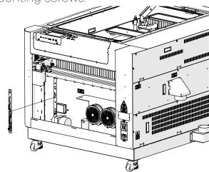
2. Install but do not fully tighten the four (4) 5/16 nuts that secure the z-axis PCB to the engraver chassis:
