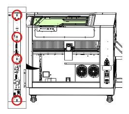
5. Connect the display port cable and the two (2) electrical harnesses to the z-axis PCB:
