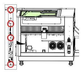
The air assist pump may need to be loosened to gain access to the bottom-most z-axis PCB nuts. Loosen the air assist pump via the four (4) Phillips screws that secure it to the bottom of the engraver.
