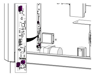
8. Loosen and remove the four (4) 5/16 nuts that secure the z-axis PCB to the engraver chassis:
