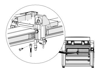
After installing a new manual focus gauge, use the auto focus feature to move the table to the calibrated focus height, then lengthen or shorten the MFG to match the focus height.
