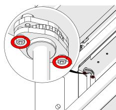
8. To adjust the table levelers, loosen the two (2) Allen screws on either side of the lead screw and twist the lead screw nut:
