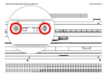
9. Once the table clamp locking screws are loosened, the table can be raised or lowered using the Allen head leveling screws shown below. Tightening the screws will lower the table and loosening the screws will raise the table:
