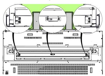
While facing the leveling adjustment points at the rear of the engraver:
