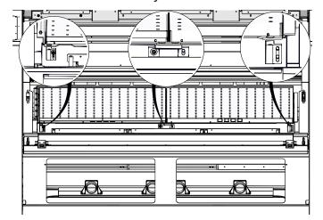
While facing the leveling adjustment points at the front of the engraver:
